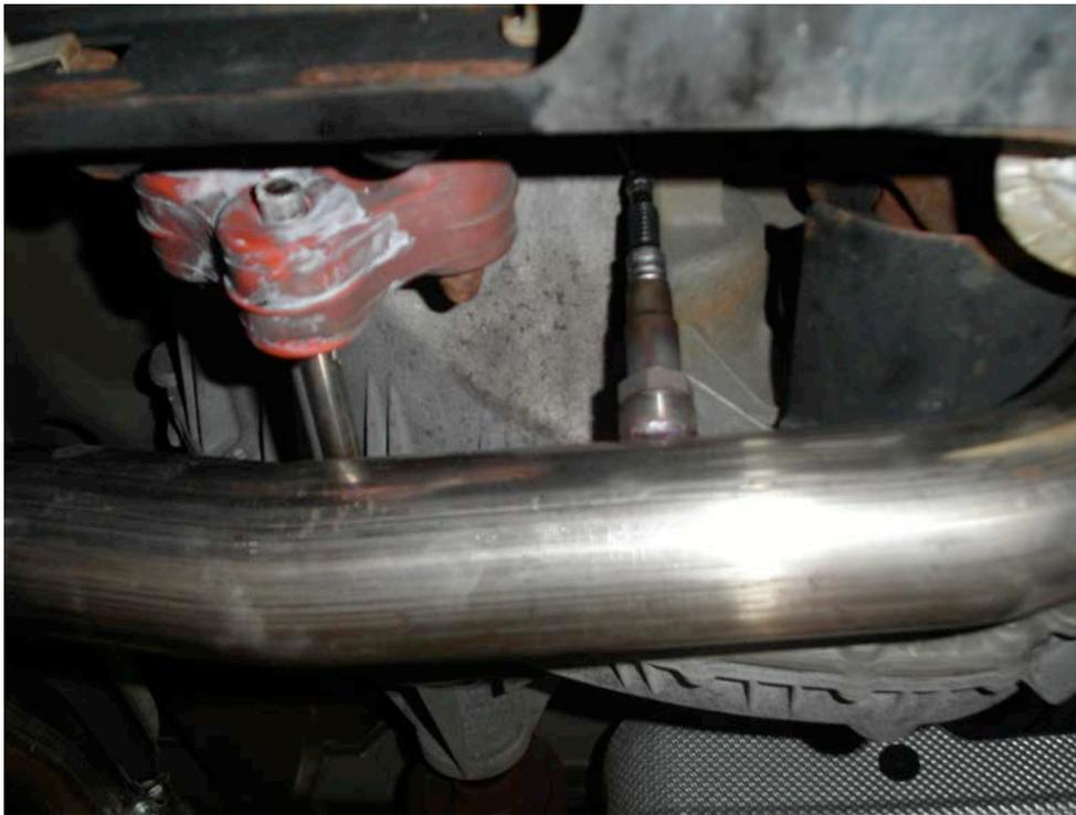
28. Install right lead pipe using 2.5 clamp, re-install right heat shield and bolt in left heat shield.
