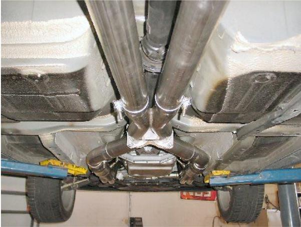
8. Install the catalytic converters (or off road pipes), the front pipes, and lastly the rear bends with the two bolt flanges welded in place. We highly recommend using red high temp RTV inside of each pipe joint. For the gasket on the two-bolt flange, we use red high temp RTV, making sure the surfaces are clean and grease free. Then assemble the joint to factory torque specs. Tighten all band clamps tight enough to prevent the pipes from rotating.
