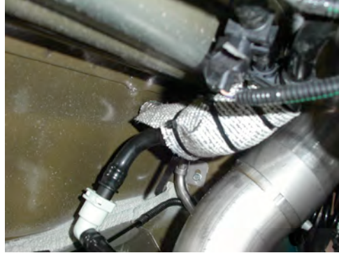
Wrapped EVAC Tube (picture #2)
