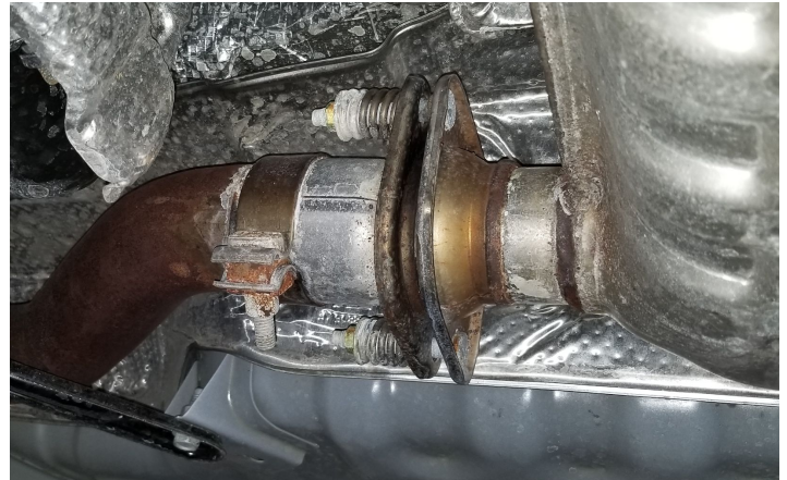
Detail 9: Flanged catback connection
