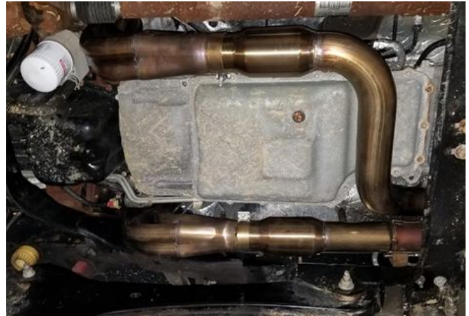
Detail 19: Headers and leads installed
