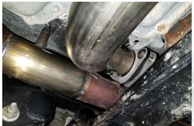
Detail 21: Catback connections (shown with SW catback)
