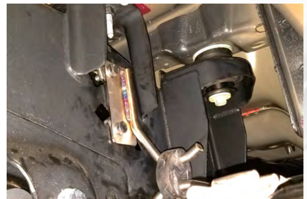
Detail 9: Frame hanger and grommet installed.
