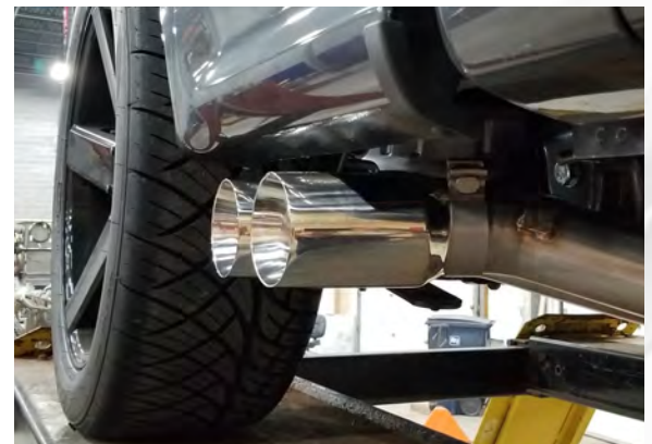
Detail 11: Tips installed.
