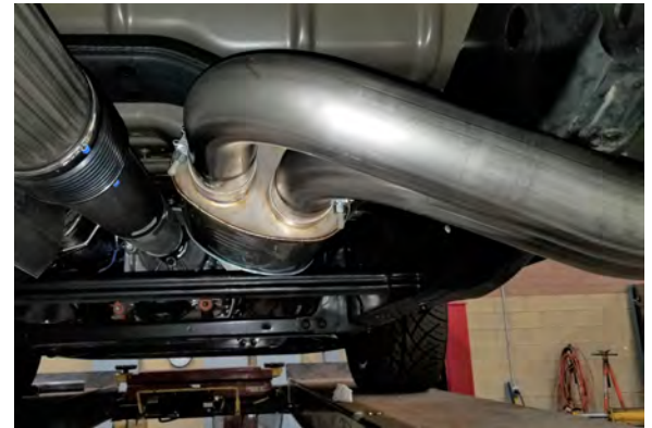
Detail 10a: Tailpipes installed to muffler.
