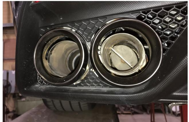
*Detail 12b: Pipe alignment/clearance in OEM tips*
