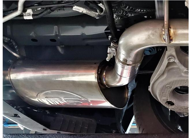
*Detail 12a: Left muffler assembly installed*
