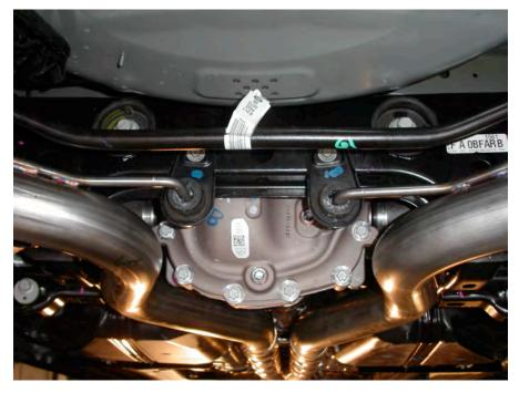
12. Reinstall rubber hangers removed from step #6 above, using (2) 8mm bolts.
