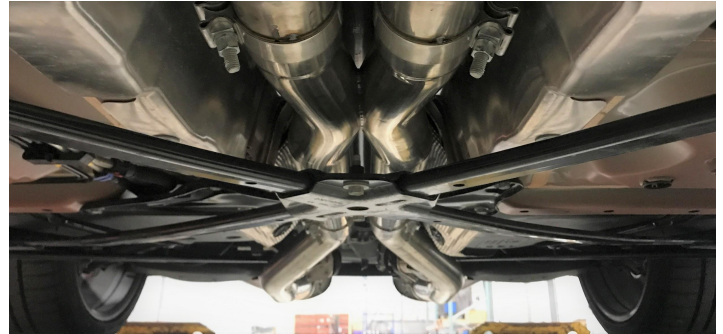
Detail 1 (X brace shown with SW system installed)
