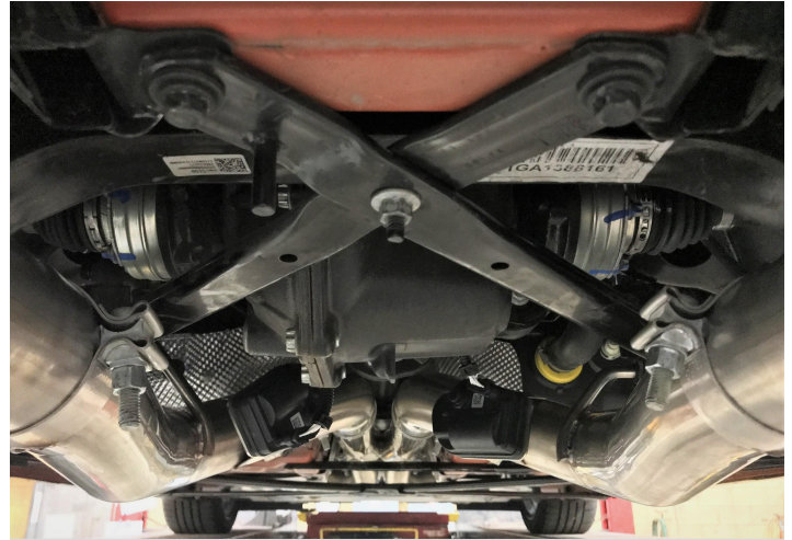
Detail 4 (X brace rear-end mount shown with SW system installed)
