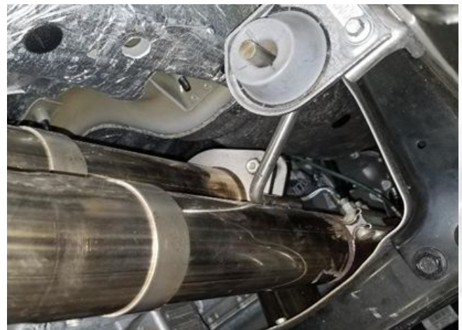
Detail 11: Inlet connection and X-pipe installed
