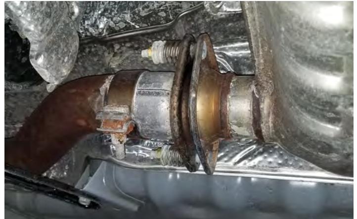
Detail 7: Flanged catback connection
