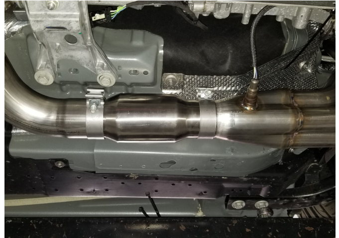
Detail 28: Lead pipes and O 2 's installed
