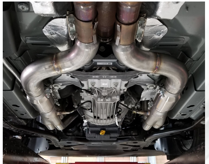
Detail 29: Catted headers installed to OEM catback connection
