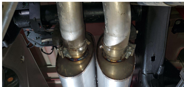
Detail 12: Hanger assemblies behind mufflers
