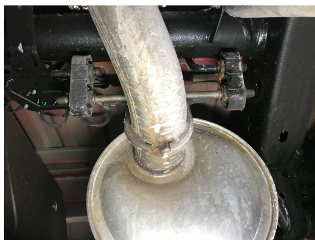
Detail 4: Rubber hangers at rear of OEM muffler
