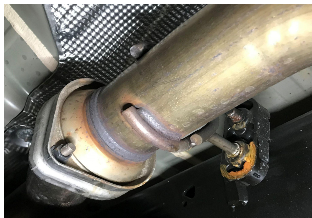
Detail 3: Factory catback connection point & rubber hanger
