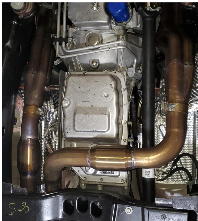
Detail 18: SW header - lead pipe connections.
