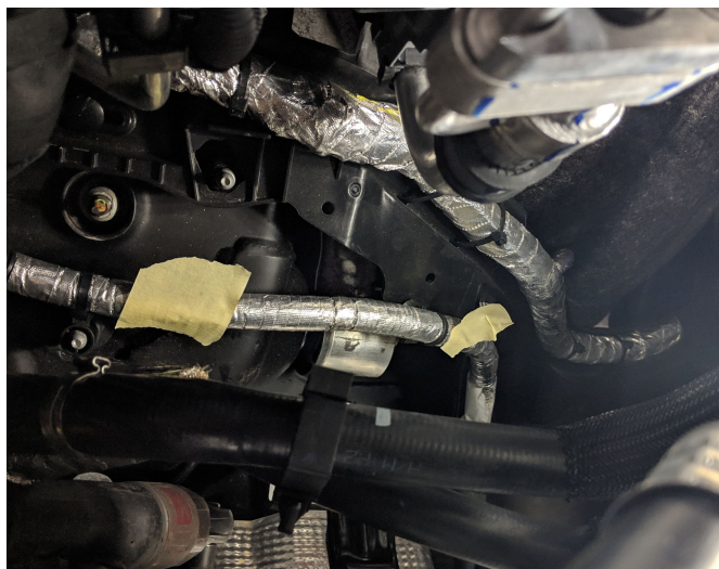
Detail 15: Wire harness to move. Locations for unhooking marked with tape.
