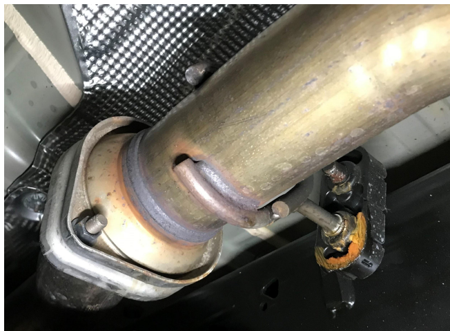
Detail 3: OEM flanged catback connection point.
