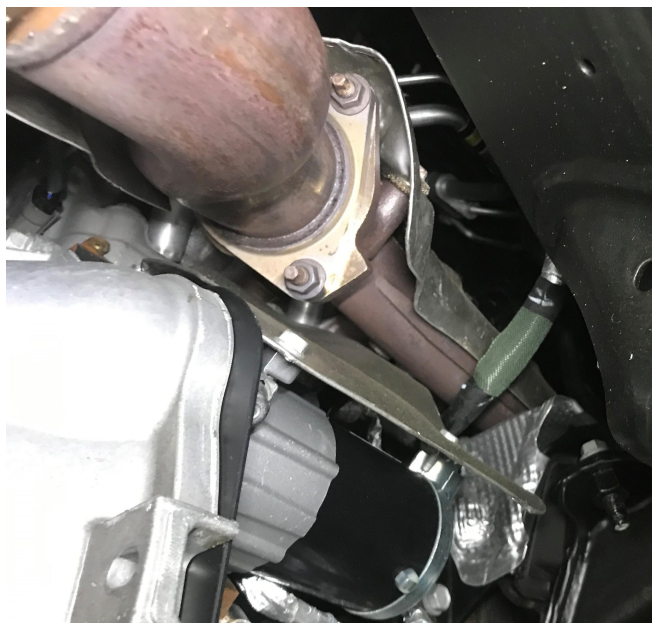
Detail 7: OEM manifold, 3 bolt flange & starter
