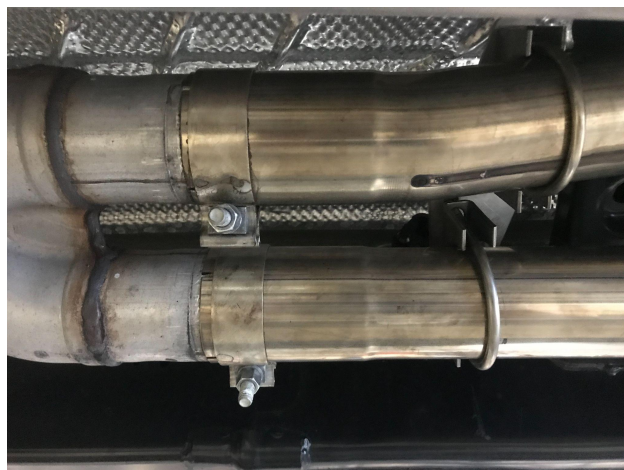
Detail 10: Muffler inlet pipes & u-bolt clamps attached to front hanger assembly.
