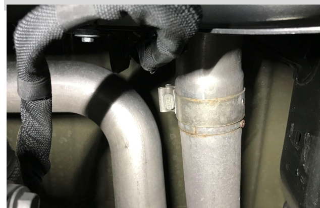
Detail 5: Passenger side OEM rear tailpipe clamp connection
