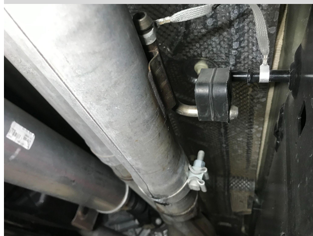
Detail 7 / 8: Front muffler hanger, grounding strap & catback clamp connection point.
