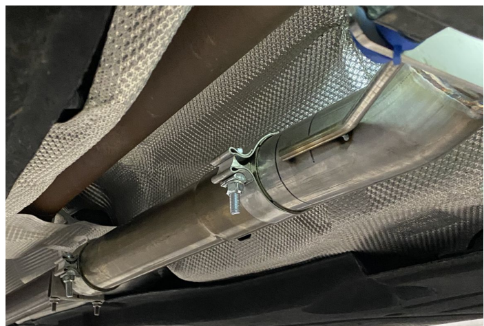
Detail 5: the tubing transition connected to the DP.
