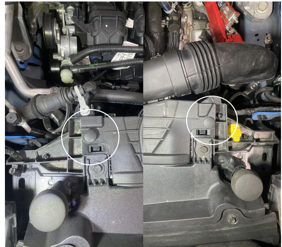
Detail 3: two push clips holding the intake duct to the core support.
