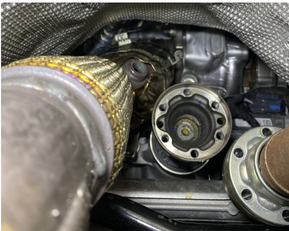
Detail 4: reference of the drive shaft unbolted and dropped for working room.
