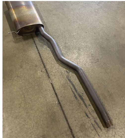
Reference picture of a properly cut factory system.
