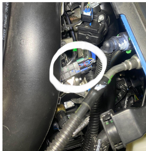
Detail 7: location of the bank one O2 sensor plug.
