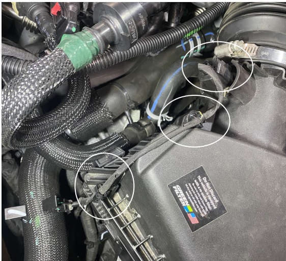
Detail 2: location of both clips and the plug.
