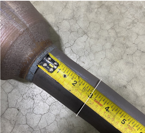
Detail 3: how to mark out your cut.
