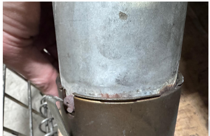
Detail 13: Metal clip to bend in order to remove tubes
