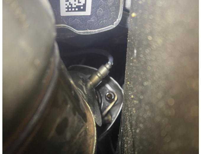
Detail 14: Heat shield will prevent you from removing O2 sensor. Remove with 10mm
