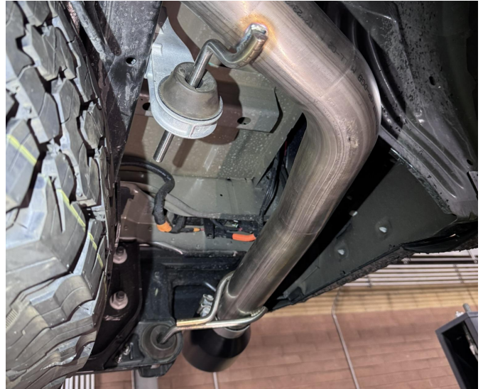
Step 20: Tails installed onto grommet
