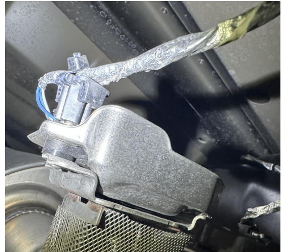
Step 3: Unplug valve motors from both sides.
