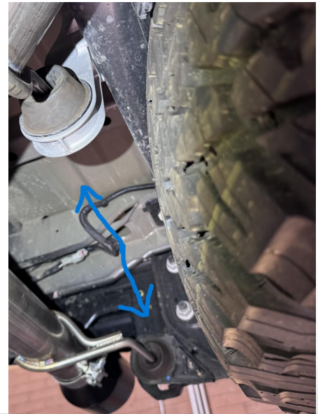
Step 8: Remove factory grommet mounts on both sides (2x10mm each)
