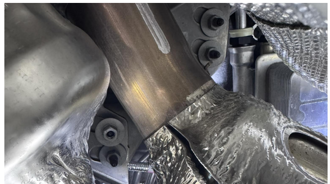
Detail 10: 4 bolts at bottom of downpipe
