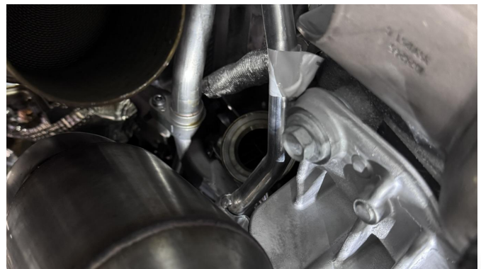
Detail 12: Wastegate location in vehicle
