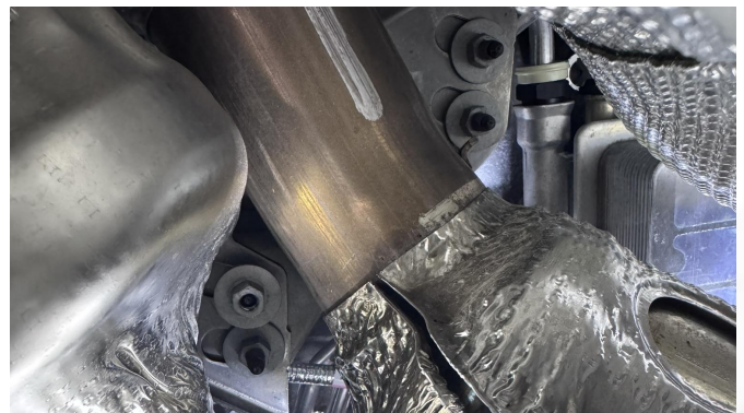
Detail 10: 4 bolts at bottom of downpipe
