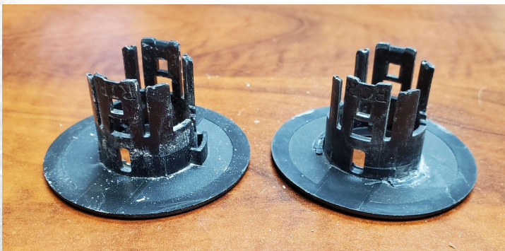
Detail A6: Remove alignment tabs
