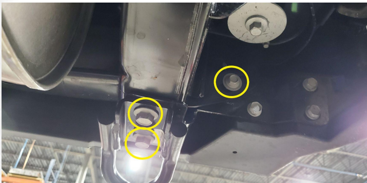
Detail A2: Remove OEM hardware
