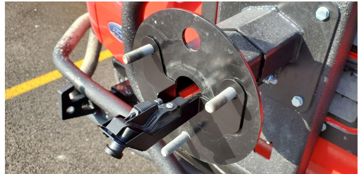
Detail 42: Camera housing installed
