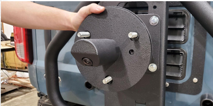
Detail 43: Camera cover installed
