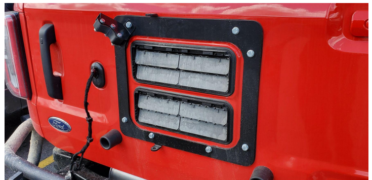
Detail 31: Tailgate plate and catch bracket installed
