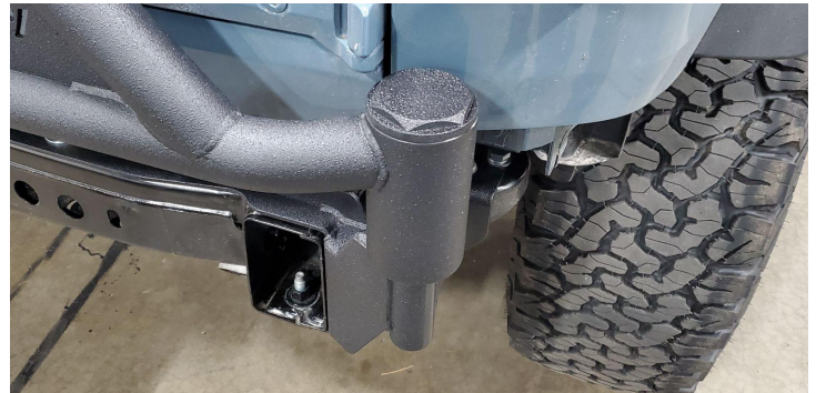
Detail 26: Spindle cap installed
