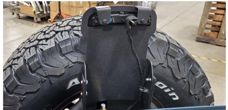
Detail 47: 3rd brake light bracket installed
