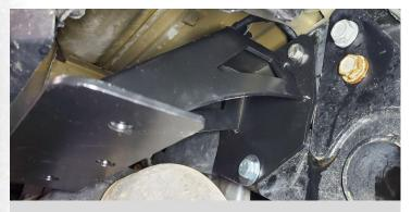
Detail A2: Install driver side mount bracket
