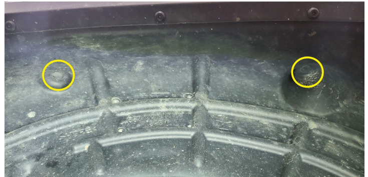
Detail A2: Remove push clips
