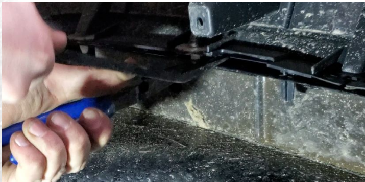
Detail A5: Remove clips and fender
