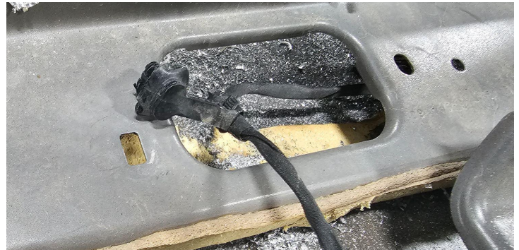
Detail A8: Disconnect harness clips
