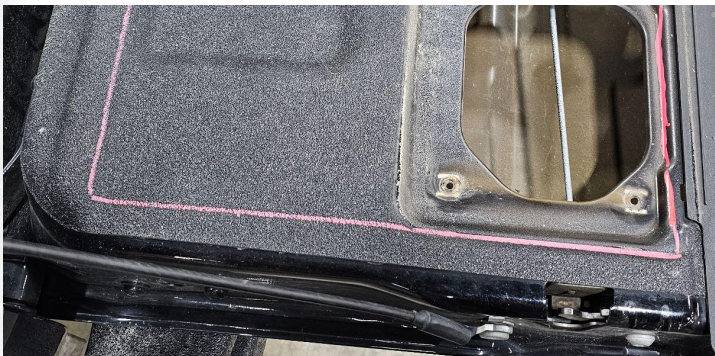
Detail A3a: Mark cut path
