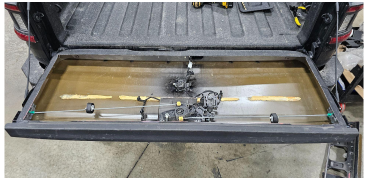
Detail A11: Clean & prep for installation
