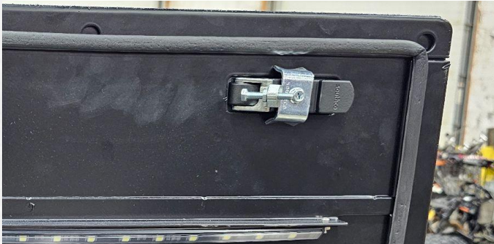
Detail B7: Latch installed
