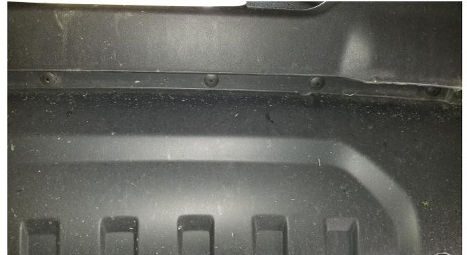
*Detail 1: Remove lower push clips*
