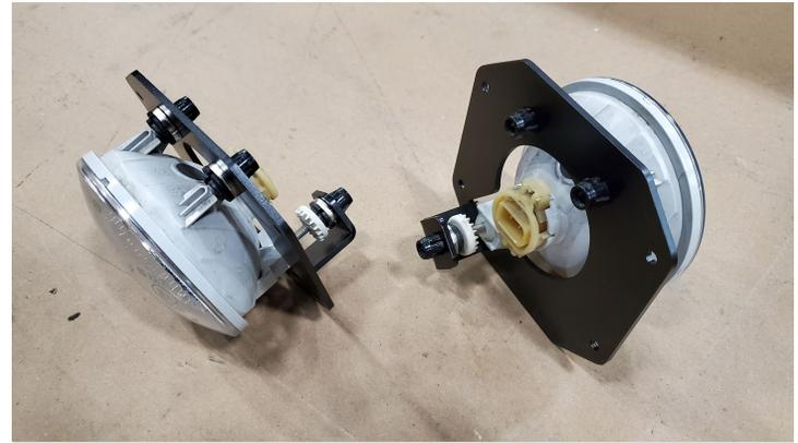
*Detail 12: Install fog lights into adapter brackets*
