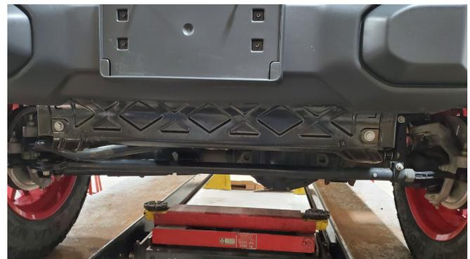
*Detail 3: Remove bolts on brace*
