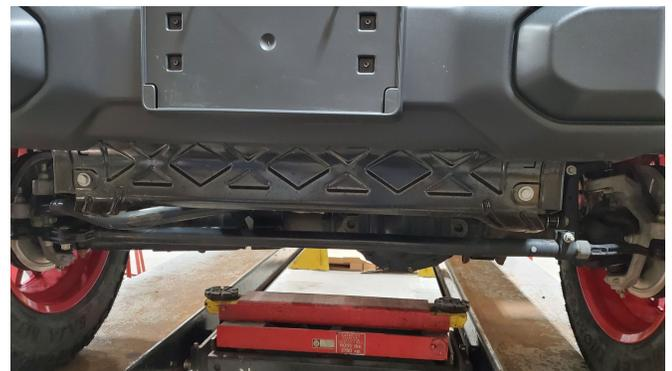
*Detail 3: Remove bolts on brace*
