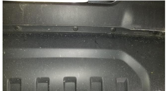
*Detail 1: Remove lower push clips*
