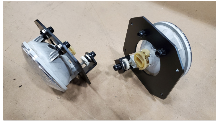
Detail 12: Install fog lights into adapter brackets
