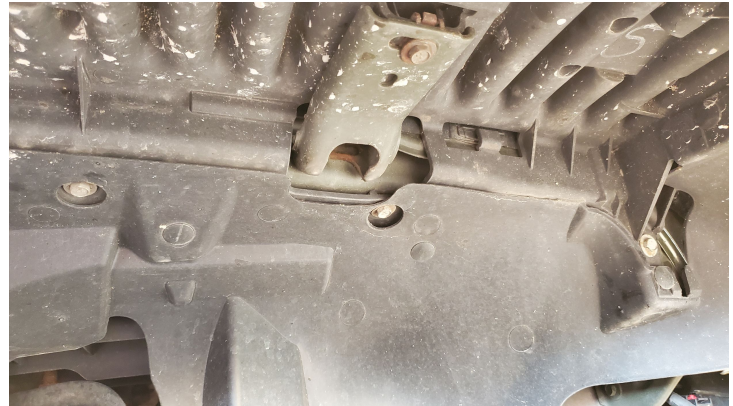
Detail 1: Remove bolts from inside fender
