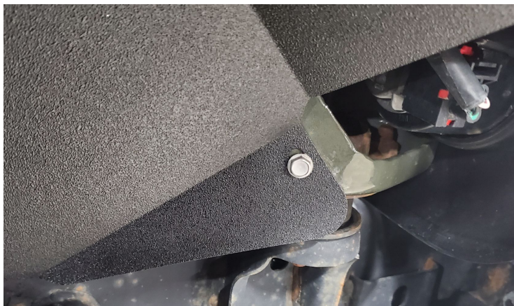
Detail 9: Install to lower mounting point
