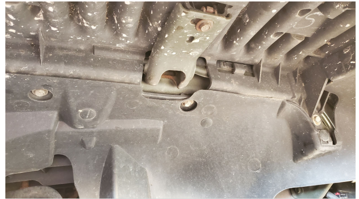
Detail 1: Remove bolts from inside fender
