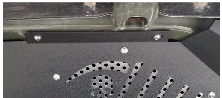
Detail 7: Install to top mounting points
