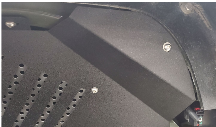
Detail 8: Install to front mounting point
