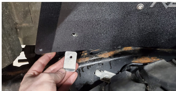
Detail 8: Install to rear mounting point using nut plate
