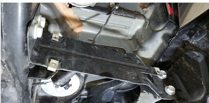
Detail A4: Remove the S-shaped bracket
