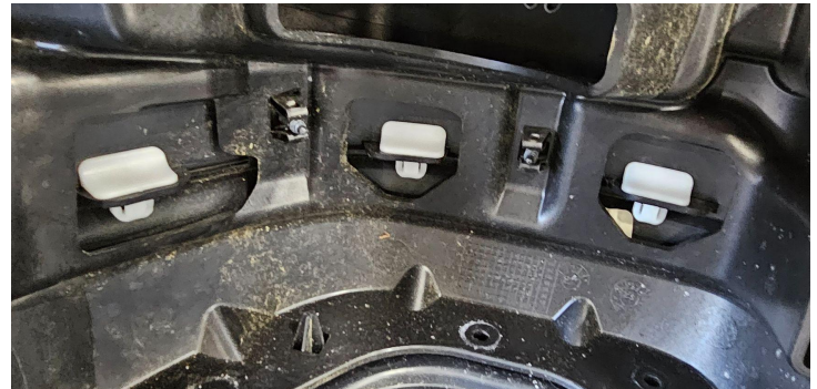
Detail A12: Remove plastic clips
