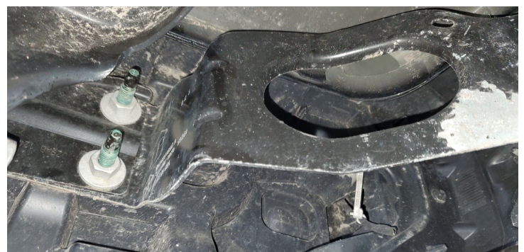
Detail A5: Remove the (2) nuts from each side
