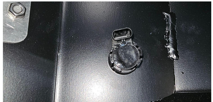
Detail B3: Install sensor mounts and sensors
