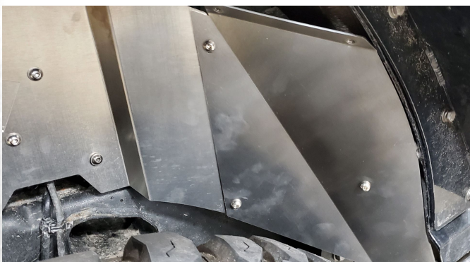
Detail 17: Front panel installed
