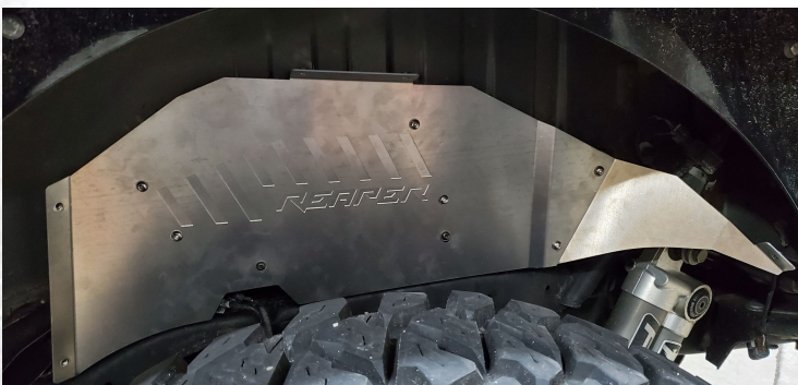
Detail 9: Logo panel and rear panel installed
