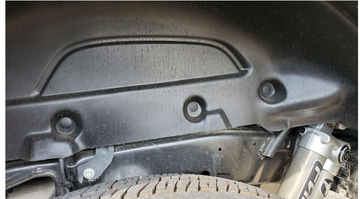
Detail 1: Remove plastic clips inside of liner.
