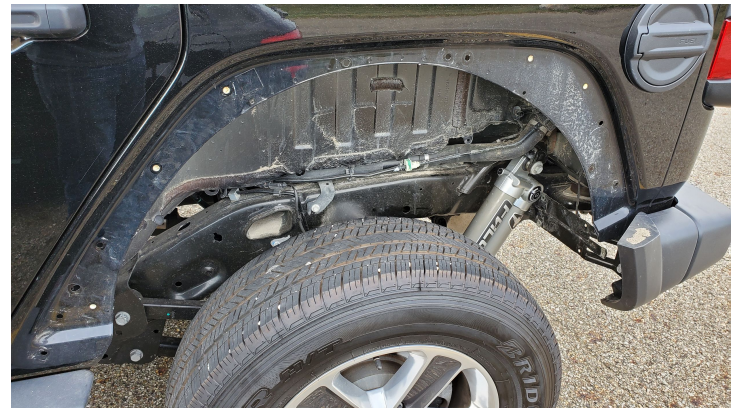
Detail 4: Fender removed.
