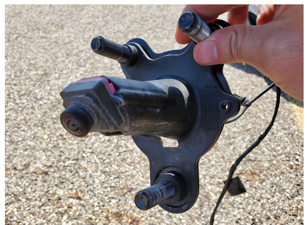
Detail 9: Remove rear camera from mount
