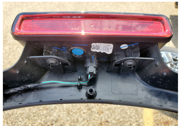
Detail 5: Remove 3rd brake light
