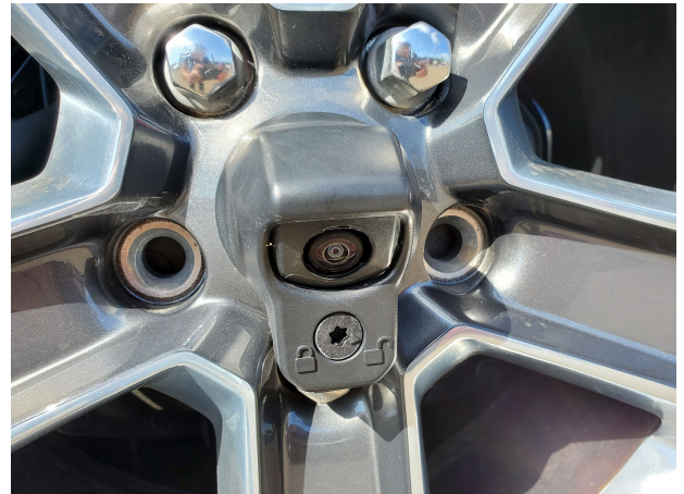
Detail 1: Remove camera cover
