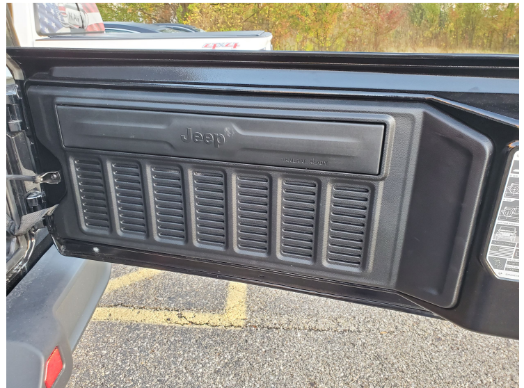
Detail 14: Remove plastic panel
