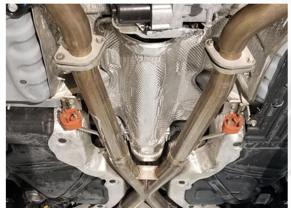
Detail 9: Inlets to X-pipe with hangers installed (shown with SW headers)
