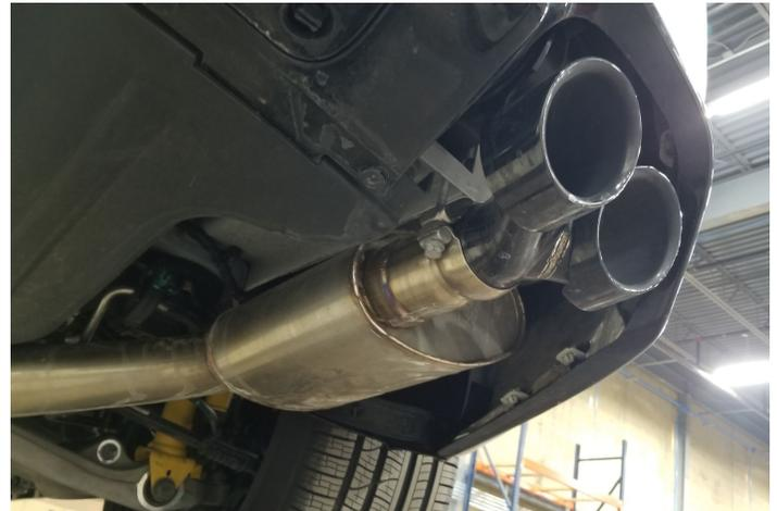
*Detail 12: Right muffler assembly with tip installed*
